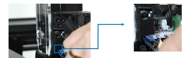
3.5 Remove the original extruder by pulling it straight up.
