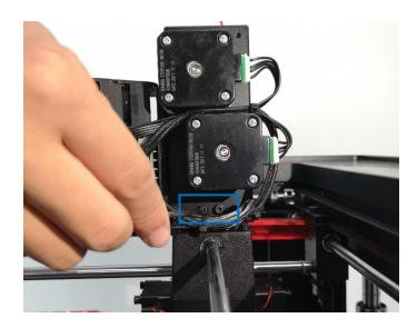
3.3 Remove the 2 screws fixing the cable chain with a 2.5mm hex wrench.
