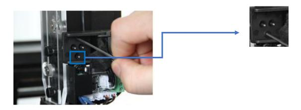
3.4 Remove the 2 screws fixing the extruder board and its origin cover with a 2.5mm hex wrench.
