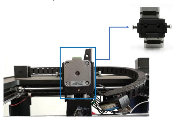
4.2 Install the original screws to the left and right (2,5mm hex wrench). Do not tighten the screws fully.
