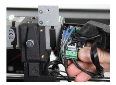
5.2 Attach the board holder. Note that the bottom screw is M2.5 and the upper one is M3.
